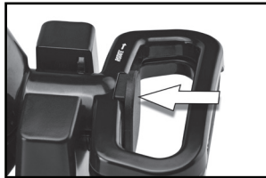
Latch in Locked Position
